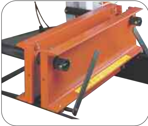
Width adjusts from 4" to over 27"; is secured with locking bolts.
