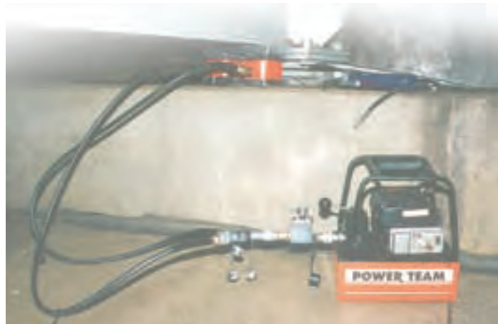
Gasoline Powered Hydraulic Pumps like this PG303 help provide hydraulic force at remote locations.
