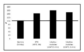
The diagram above shows the tensile shear strength of Al/Al bonding after sterilization expressed as % from the initial value. The specimens were cured by exposure to 80 °C for approximately 20 min.
