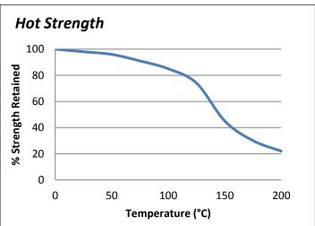
"Hot strength" shear strength tests performed on mild steel. Fully cured then conditioned to pull temperature for 30 minutes before testing. ES558 can withstand higher temperatures for brief periods (such as for paint baking and wave soldering processes) providing the joint is not unduly stressed. The minimum temperature the cured adhesive can be exposed to is -40°C (-40°F) depending on the materials being bonded.
