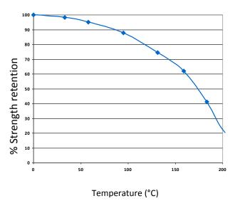
ES5722 can withstand higher temperatures for brief periods (such as for paint baking and wave soldering processes) providing the joint is not unduly stressed. The minimum temperature the cured adhesive can be exposed to is -40°C (-40°F) depending on the materials being bonded.
