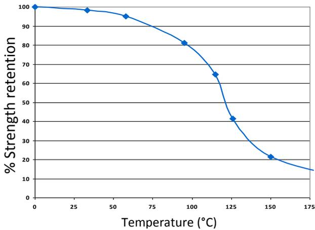
TA4310 can withstand higher temperatures for brief periods (such as for paint baking and wave soldering processes) providing the joint is not unduly stressed. The minimum temperature the cured adhesive can be exposed to is -40°C (-40°F) depending on the materials being bonded.
