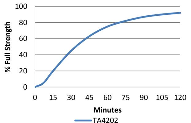
Graph shows typical strength development of bonded components at 23°C. An increase of 8°C in temperature will halve the cure time. Lower temperatures will result in a slower cure time.
