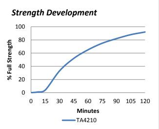
Graph shows typical strength development of bonded components at 23°C. An increase of 8°C in temperature will halve the cure time. Lower temperatures will result in a slower cure time.
