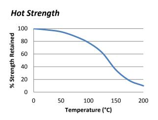
"Hot strength" shear strength tests performed on mild steel. Fully cured specimens conditioned to pull temperature for 30 minutes before testing at temperature. TA4210 can withstand higher temperatures for brief periods (such as for paint baking and wave soldering processes) providing the joint is not unduly stressed. The minimum temperature the cured adhesive can be exposed to is -40°C (-40°F) depending on the materials being bonded.
