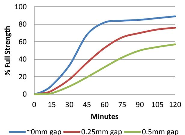
Graph shows typical strength development of bonded components at 23°C. An increase of 8°C in temperature will halve the cure time. Lower temperatures will result in a slower cure time.
