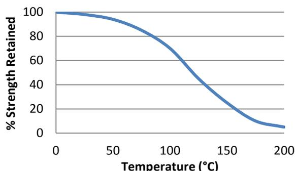
"Hot strength" shear strength tests performed on mild steel. Fully cured specimens conditioned to pull temperature for 30 minutes before testing at temperature. TA436 can withstand higher temperatures for brief periods (such as for paint baking and wave soldering processes) providing the joint is not unduly stressed. The minimum temperature the cured adhesive can be exposed to is -55°C (-65°F) depending on the materials being bonded.
