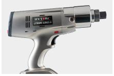
The nickel plated all-aluminum housing greatly improves corrosion resistance and overall durability. The all new 36V brushless motor has more than 5 times longer life than its predecessor. Gearboxes are redesigned for 20% greater strength and reliability. The integrated rear cover shock guard absorbs impact protecting the display and buttons. Hall Effect trigger and directional switches increases dependability.
