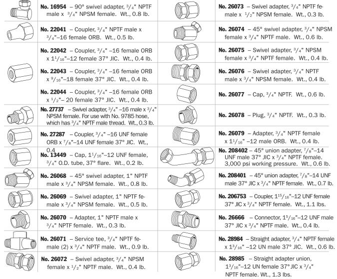
NOTE: The recommended maximum working pressure on the above fittings is 5,000 psi except the 208402.
