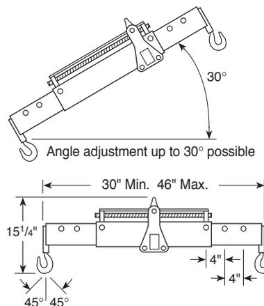
The working length is adjustable in three positions from 30" to 46". Maximum chain angle is 45°.
