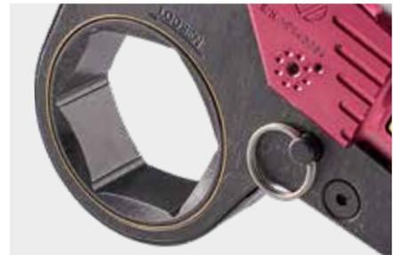
The XLCT is available with interchangeable cartridges for 6-point hex, 12-point hex, allen drives, square drives, open spanners, and many other configurations to simplify the most challenging bolting jobs.
