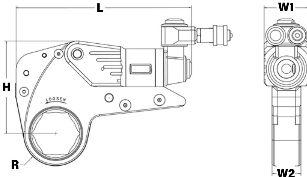
LEGEND: H = HEIGHT W1 = WIDTH OF POWERHEAD W2 = WIDTH OF LINK L = LENGTH R = RADIUS
