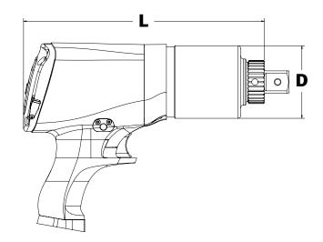
**LEGEND: H** = HEIGHT **W** = WIDTH **L** = LENGTH **D** = OUTER DIAMETER OF GEARBOX
