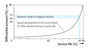
The dirt load collected in a filter element gradually increases during service, which also leads to a higher pressure drop. The resulting vacuum or back pressure is monitored by a clogging indicator. Once a preset value is reached, an electrical and/or optical signal is generated.
