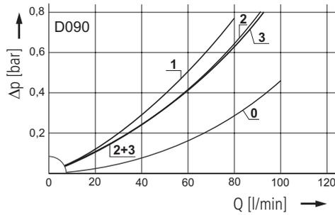
Pressure drop as a function of the **kinematic viscosity**
