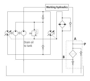
This circuit layout has the advantage that drain oil pressures are comparatively low.
